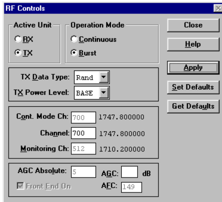
Figure 23: PCN TX tuning window 1
